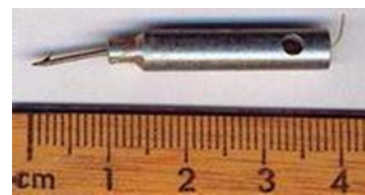
ACTUAL SCALE / SIZE: Barb is a straight #8 fishhook with a length of 4mm and the entire dart length is less than 1 cm.
